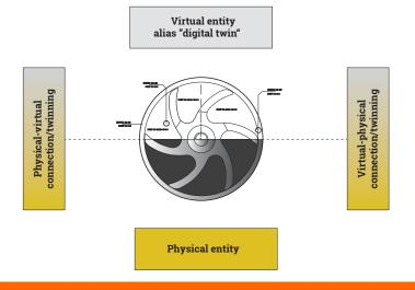
The Digital Twin ...can be a businesses, processes, or machines. ...should contain the current and past state, ...can help us capture and formalize knowhow and ...should link different lifecycle phases.
